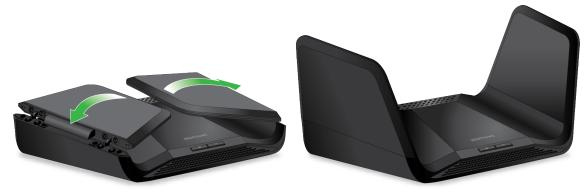
Figure 5. Position the antennas
