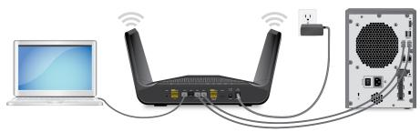
Figure 8. Ethernet port aggregation to a LAN device
