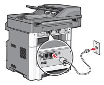
Faxing 126 **3** Remove the plug from the printer EXT port  $\widehat{\blacksquare}$ .
