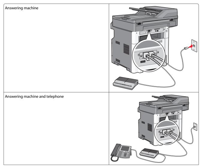
Telephone or a telephone with an integrated answering machine
