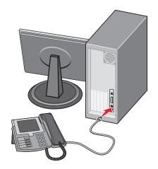
**5** Connect an additional telephone cord (not provided) from the computer modem to the printer EXT port  $\widehat{\blacksquare}$ .
