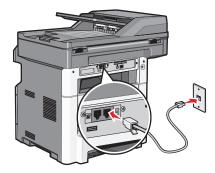
**3** Remove the protective plug from the printer EXT port  $\widehat{\blacksquare}$ .
