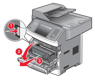
**2** Lift the flap at the front of the printer, and then remove any jams.
