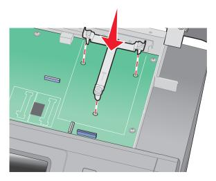
**6** Install the ISP onto the plastic tee. Angle the ISP over the plastic tee, and then approach the plastic tee so that any overhanging connectors will pass through the ISP opening in the system board cage.
