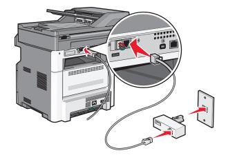
**3** Connect the answering machine or telephone to the adapter. Use one of the following methods:
