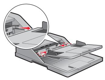
**2** Pull out the jammed paper by pulling the sheet on the bottom.
