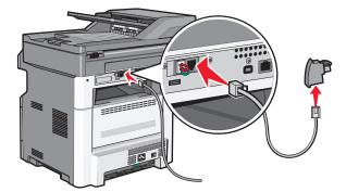
Faxing 130 **3** Connect the adapter into the N slot of an active analog telephone wall jack.
