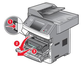
**4** Lift the flap at the front of the printer, and then remove any jammed sheets.
