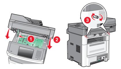
**Warning—Potential Damage:** Make sure the system board is locked to prevent possible damage to the printer if it is moved.
