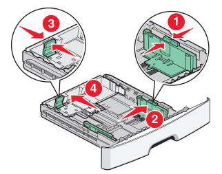
For long paper like A4 or legal, squeeze and slide the length guide backwards to accommodate the length of paper you are loading.
