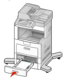
**8** If a different type of paper was loaded than the type previously loaded in the tray, then change the Paper Type setting for the tray from the printer control panel.
