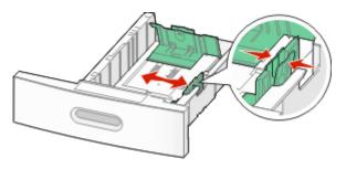
**3** Unlock the length guide, squeeze the length guide tab inward as shown, and slide the guide to the correct position for the paper size being loaded.
