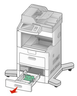
2 Squeeze the width guide tab inward as shown, and move the width guide to the correct position for the paper size being loaded
