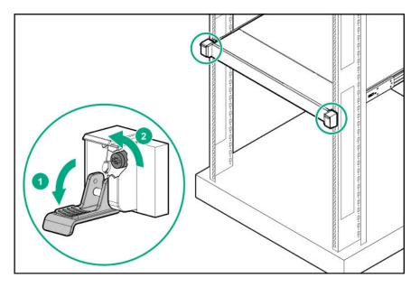
**3.** Extend the server on the rack rails until the server rail-release latches engage.
