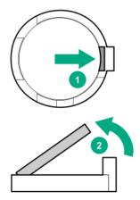
9. Insert the battery with the "+" side facing up on the socket, and then press the battery down to secure it in place.
