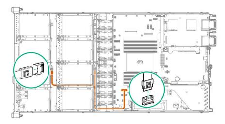
• 8 LFF SAS/SATA (box 1 and 2) connected to HPE Smart Array type-a modular controller
