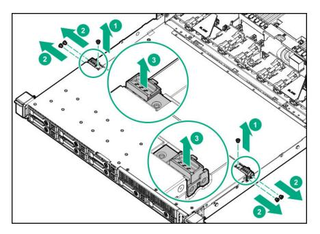
**14.** Remove the outer drive cage.
