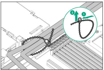
Install the inner drive cage blank.
