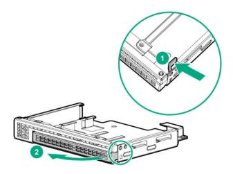
**10.** Install the ODD into the cage.
