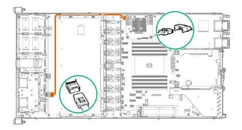
2SFF SAS/SATA/uFF drives installed in outer cage (box 2) and connected to type-p storage controller This illustration shows the cabling for type-p storage controller installed in slot 2. The cabling for type-p storage controller installed in slot 3 is similar.
