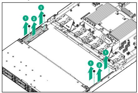
**13.** Remove the drive cage latches.
