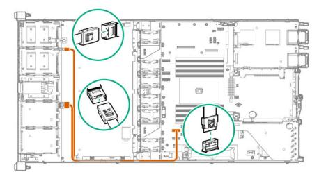
8 SAS/SATA drives (box 1) connected to HPE Smart Array type-a modular controller
