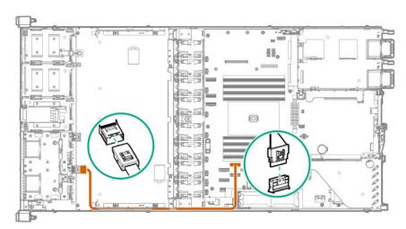
• 2SFF SAS/SATA/uFF drives installed in outer cage (box 2) and connected to type-a storage controller
