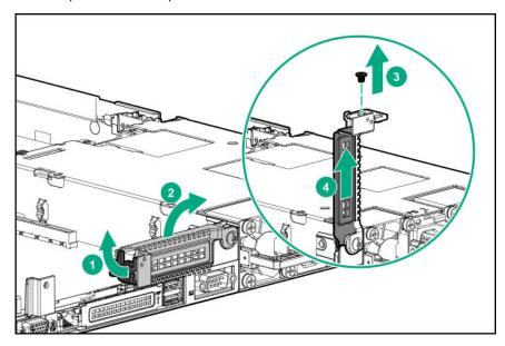
Secondary riser slot 3: full-height blank
