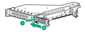
Secondary riser slot 3: low-profile blank
