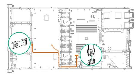
4 LFF SAS/SATA (box 1) connected to HPE Smart Array type-a modular controller
