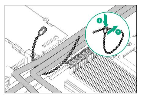
**10.** Remove the inner drive cage blank.
