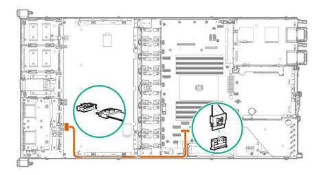
2 + 2NVMe drives installed in outer and inner cages (box 2 and 4) and connected to system board (For 16SFF SAS/ SATA + 4NVMe configuration)
