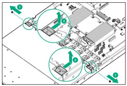
**10.** Remove the inner drive cage.
