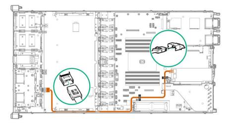
2SFF SAS/SATA/uFF drives installed in outer and inner cages (box 2 and 4) and connected to system board
