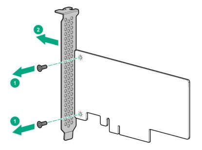
**b.** Install the low-profile bracket on the expansion board.
