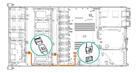
2SFF SAS/SATA drives installed in outer and inner cages (box 2 and 4) and connected to type-p storage controller
