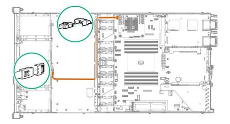
• 8 LFF SATA (box 1 and 2) connected to system board
