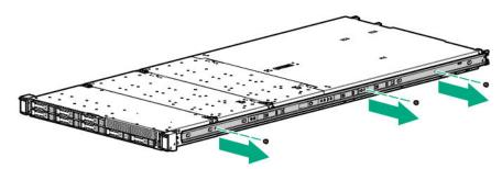
**7.** Slide the inner rails towards the front of the chassis and pull them out.
