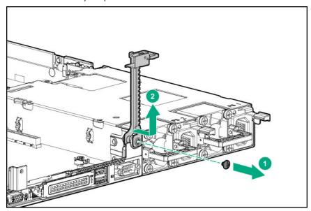
**12.** Install the full-height PCIe bracket.
