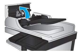
Remove any visible lint or dust from each of the feed rollers and the separation pad using compressed air or a clean lintfree cloth moistened with warm water.
