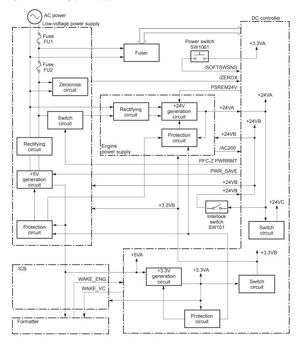
The low-voltage power supply converts the AC power into three DC voltages, which it then subdivides, as described in the following table.
