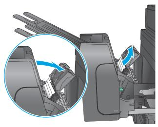
4. Open the jam-access door. If jammed paper is visible inside the jam-access door, pull it straight up to remove it.
