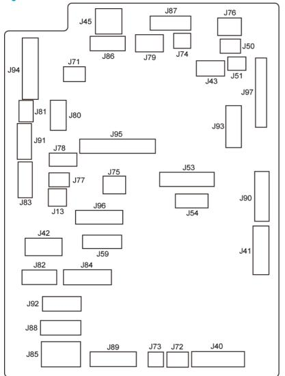
Figure 2-48 DC controller PCA connectors
