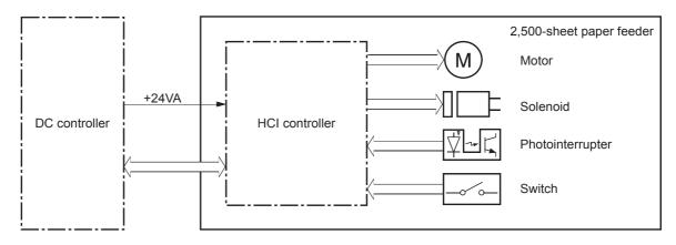
Figure 1-50 Pickup and feed components (2,500-sheet high-capacity paper feeder)
