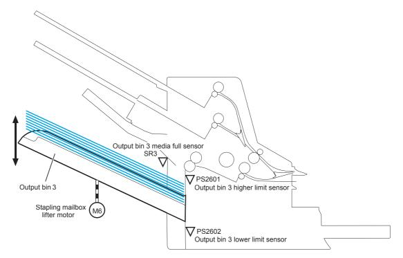
The operational sequence of the output bin 3 lift operation is as follows:
