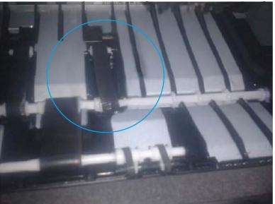
Figure 2-66 Paper feed assembly belt
