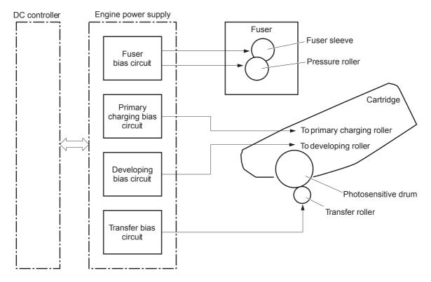
The primary charging bias is used to charge the surface of the photosensitive drum evenly to prepare for image formation. The primary charging bias circuit generates the bias.
