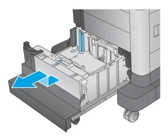
5. If jammed paper is in the feed area, pull it down to remove it.
