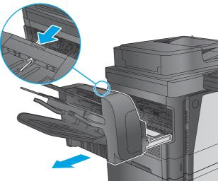
2. M630z (or other models if the stapling mailbox is installed): Press the button to release the stapling mailbox, and remove it from the product.
