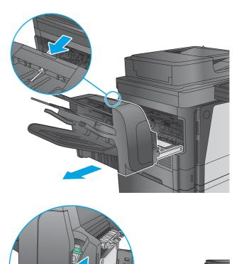
2. Press the latch to release the stapler door.
