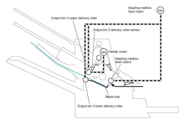
The stapling mailbox controller determines an output bin 3 upper delivery roller failure and notifies the formatter through the DC controller when it does not detect the output bin 3 upper delivery roller sensor for a specified period of time after the paddle motor starts rotating.
