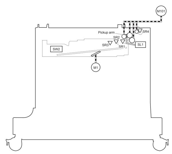
Figure 1-48 Pickup and feed components (1x500-sheet paper feeder with cabinet)
