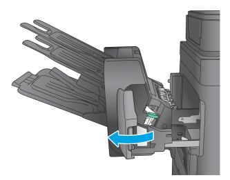
**4.** Lift the green tab on the staple cartridge up, and then pull the staple cartridge straight out.
