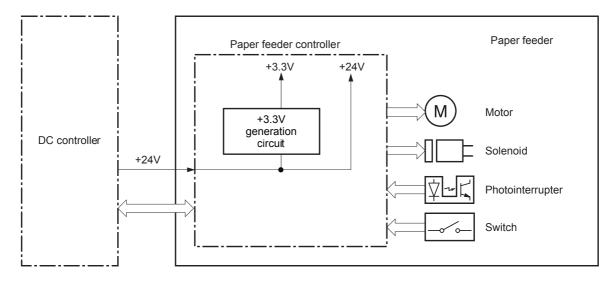
Figure 1-46 Pickup and feed components (1x500-sheet paper feeder)
