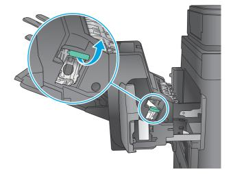
5. Lift up on the small lever at the back of the staple cartridge.
