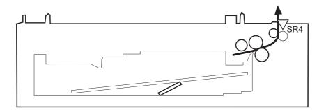
Figure 1-54 1x500-sheet paper feeder with cabinet media feed sensor
