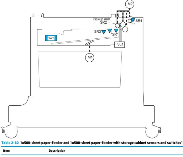
**Figure 2-69** 1x500-sheet paper-feeder and 1x500-sheet paper-feeder with storage cabinet sensors and switches<sup>1</sup>
