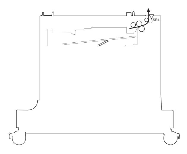
Figure 1-55 2,500-sheet high-capacity paper feeder media feed sensors
