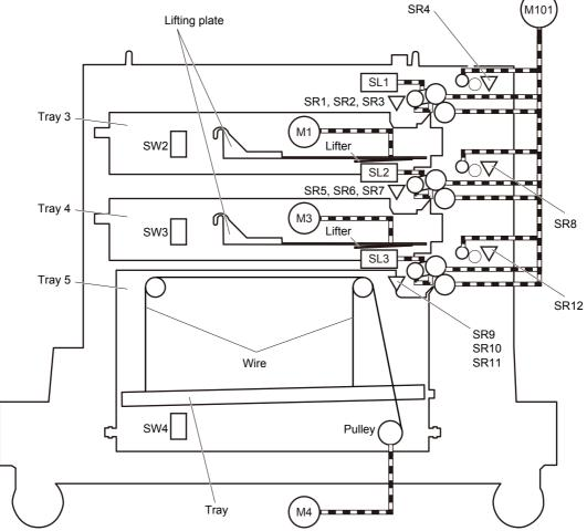
Table 2-18 Sensors (2,500-sheet high-capacity feeder) (HCI)
