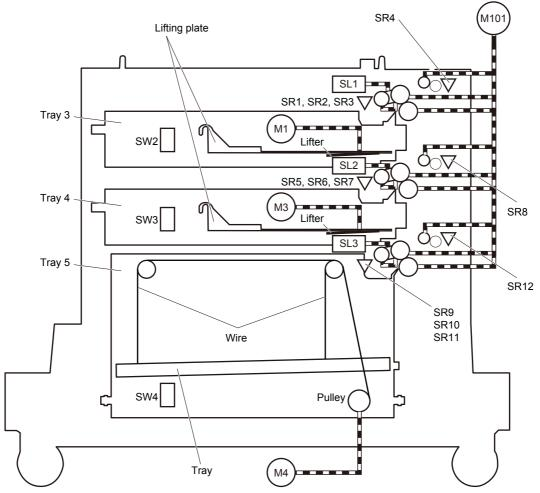
Figure 2-70 2,500-sheet high-capacity feeder (HCI) sensors and switches
