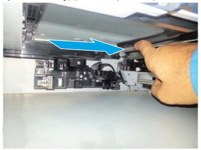
This area is above tray 2 pickup roller assembly. The arrow indicates duplex refeed path.
