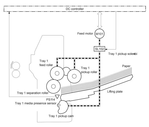
The operational sequence of picking one sheet of paper from Tray 1 is as follows:
