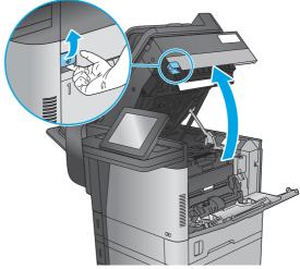
3. If the paper is difficult to remove, or if no jammed paper is visible in Tray 1, lift the top-cover-release latch and open the top cover.
