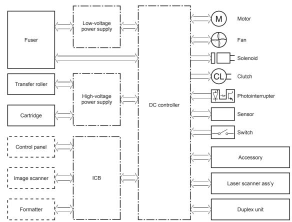
Figure 1-4 DC controller block diagram
