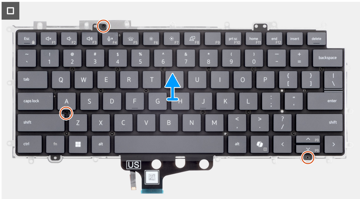
Figure 87. Removing the keyboard
