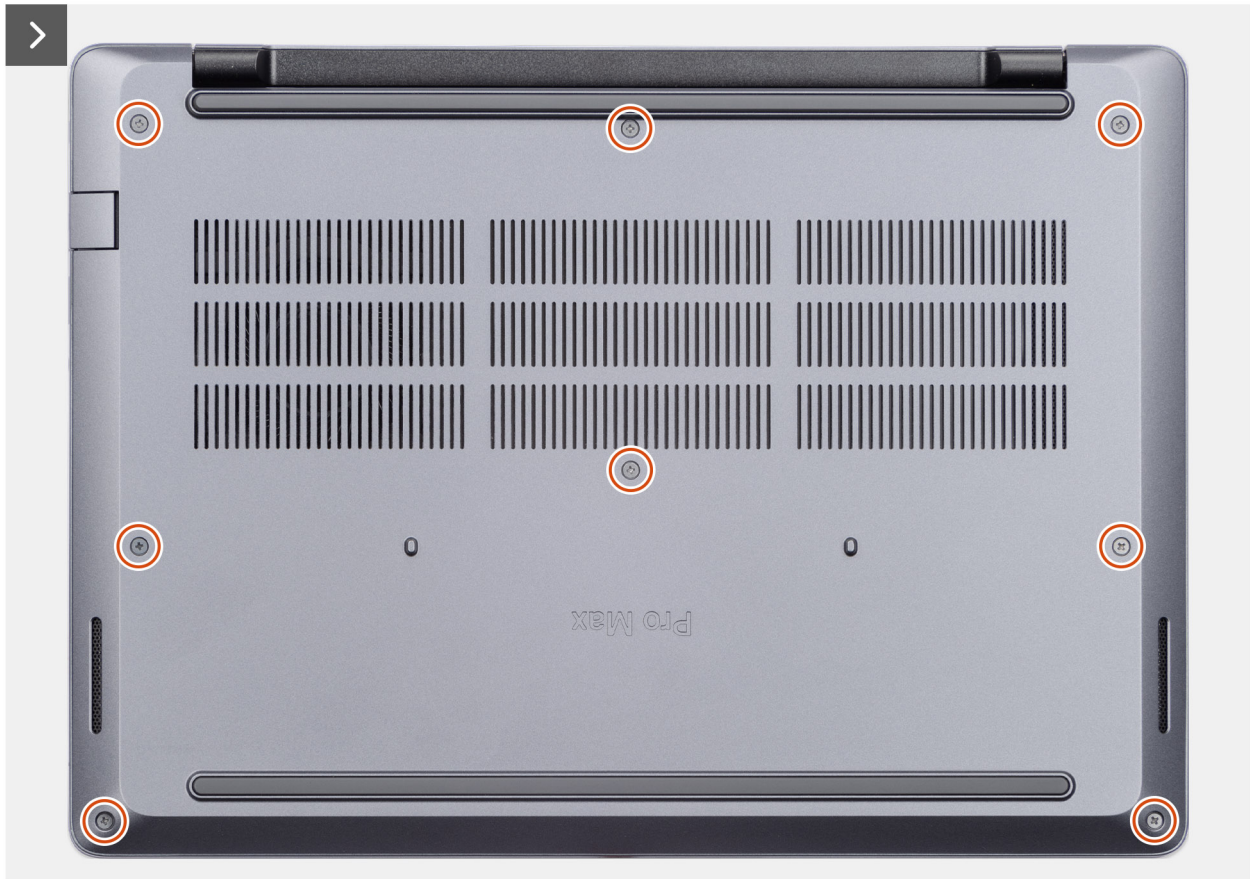
Figure 11. Removing the base cover
