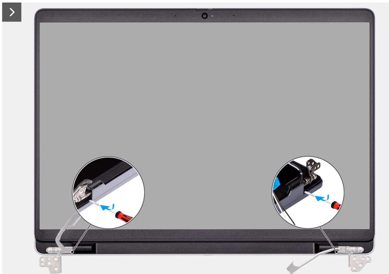
Figure 49. Removing the display bezel
