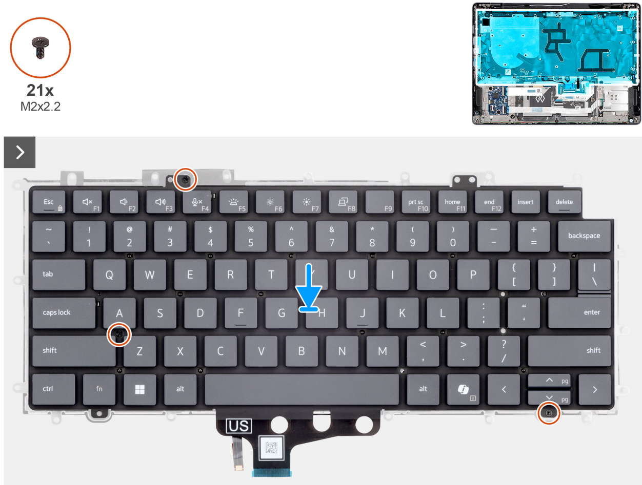
Figure 88. Installing the keyboard
