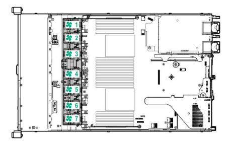
The loss of a single fan rotor (one standard fan) causes loss of redundancy. The loss of two fan rotors (2 standard fans or 1 high-performance fan) causes the server to initiate a shut down.
