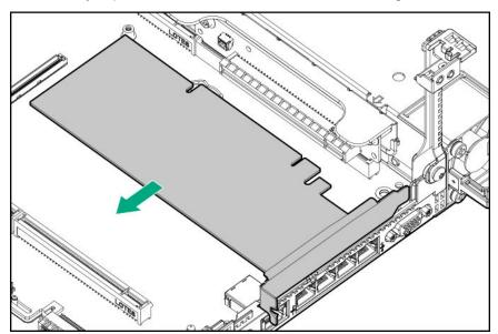
10. Remove the PCI riser cage.
