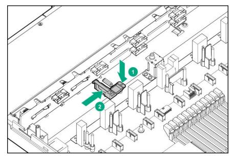
Slide the energy pack into the left retainer, and then install the right retainer.
