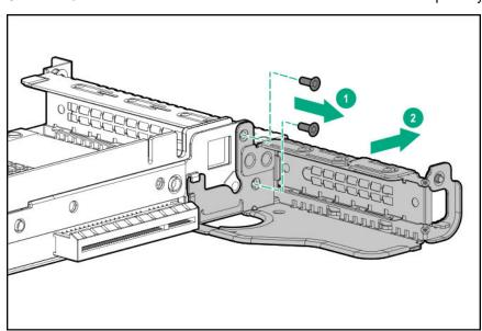
If installed, remove the low-profile riser cage.
