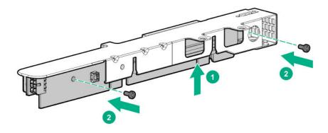
**10.** Install the drive cage on the riser cage.
