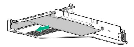
8. Remove the existing riser board from the PCI riser cage.
