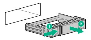
3. Press the Do Not Remove button to open the release handle.
