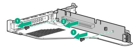
**9.** Install the optional riser board in the riser cage.
