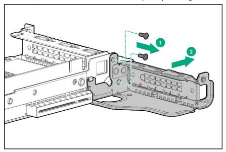
If needed, install the riser board removed in step 7 on the rear drive riser cage bracket.
