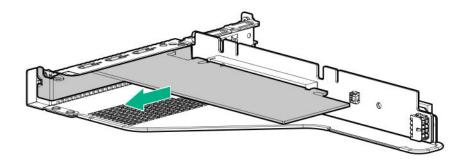
7. Remove the existing riser board from the riser cage.
