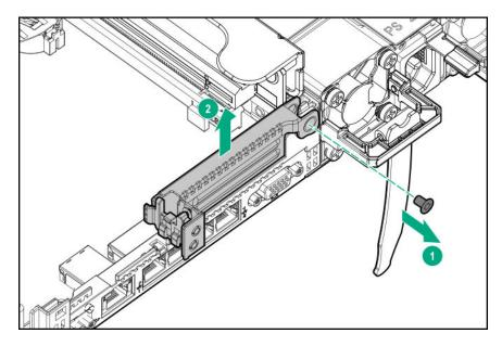
9. Install the full height PCIe x16 riser cage latch.Use a T-15 Torx screwdriver to remove the riser cage screw.
