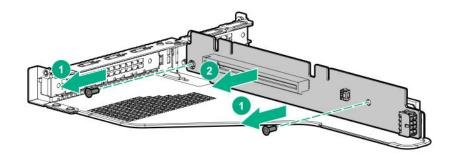
If installed, remove the slot 2 bracket from the primary riser cage.
