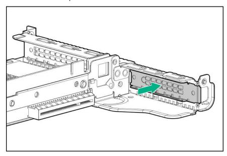
Use a Torx T-10 screwdriver to install the controller.
