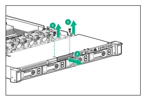
Install the 4 LFF display port/USB module.
