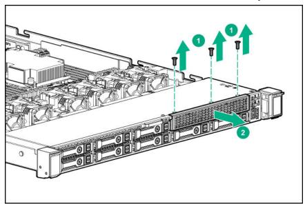
Use a T-10 Torx screwdriver to install the 2 SFF NVMe drive cage.
