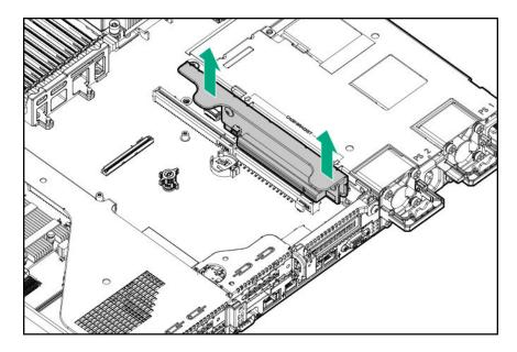
8. Lift and remove the secondary riser cage latch.Use a T-15 Torx screwdriver to remove the riser cage screw.
