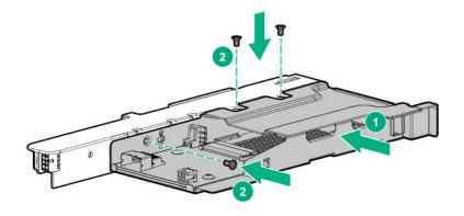
**11.** If needed, install the riser cage bracket on the rear drive riser cage.
