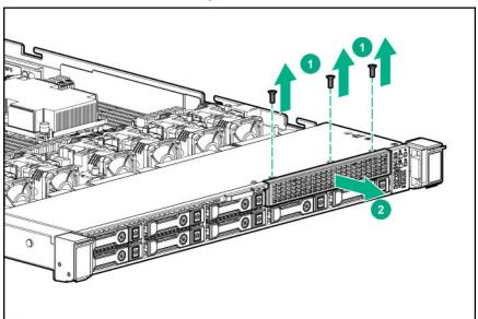
Install the 8 SFF display port/USB/optical blank option.
