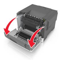
**2** Slide the release button on the right side of the printer, and then open the top door.
