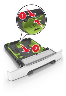
**Note:** Use the size indicators on the bottom of the tray to help position the guide.
