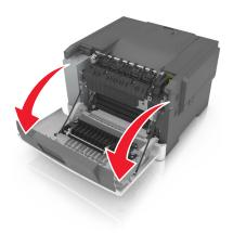
**2** Slide the release latch on the right side of the printer, and then open the top door.
