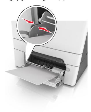
5 From the printer control panel, touch to clear the message and continue printing. For non-touch-screen printer models, select Next > OK > Clear the jam, press OK > OK.
