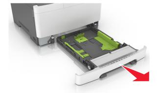
2 If the paper is longer than letter-size paper, then push the length guide tab at the back of the tray to extend it.
