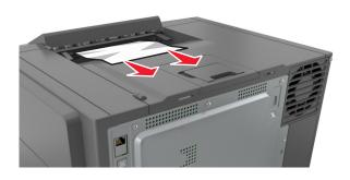
2 From the printer control panel, touch to clear the message and continue printing. For non-touch-screen printer models, select Next > Clear the jam, press OK, and then press of to confirm.
