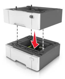
4 Align the printer with the 650-sheet duo tray, then lower the printer into place.
