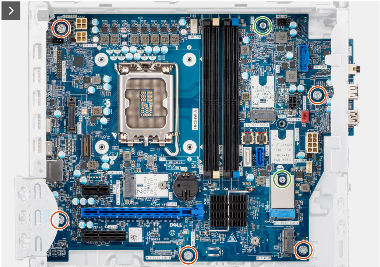
Figure 89. Installing the system board
