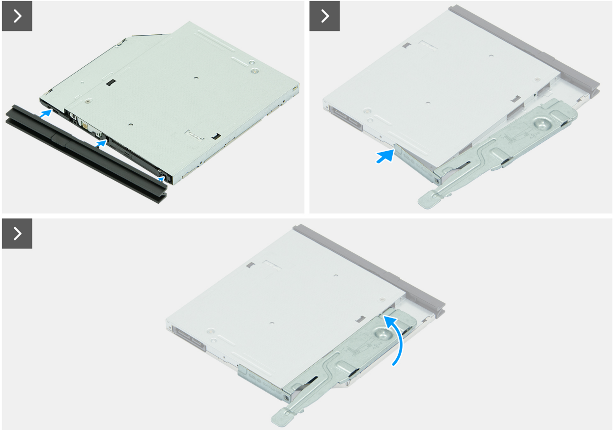
Figure 19. Installing the optical drive
