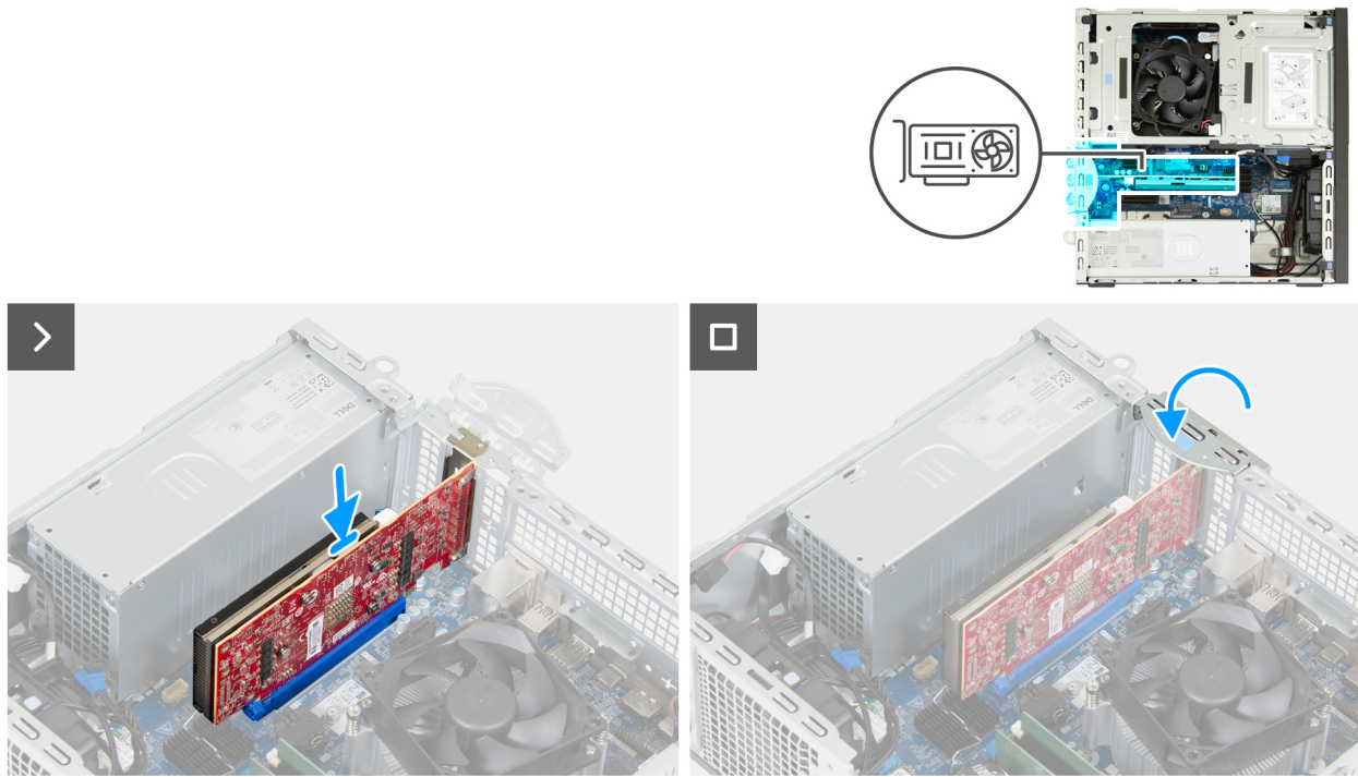
Figure 40. Installing the graphics card
