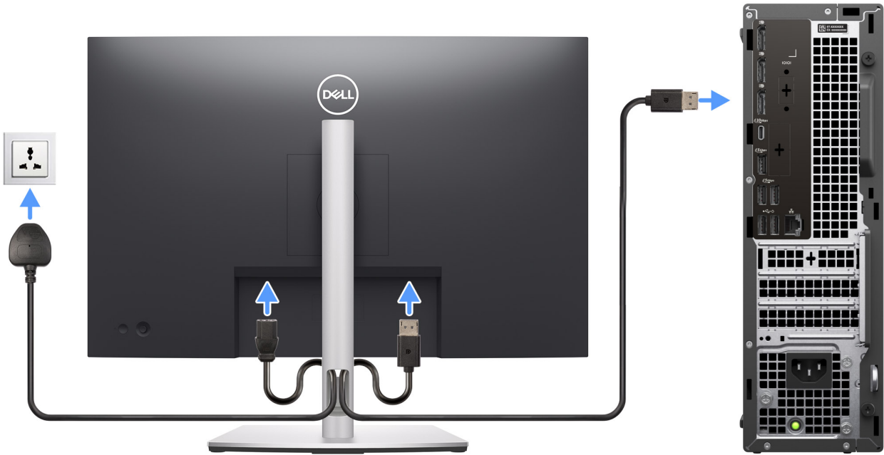
Figure 5. Connecting the display
