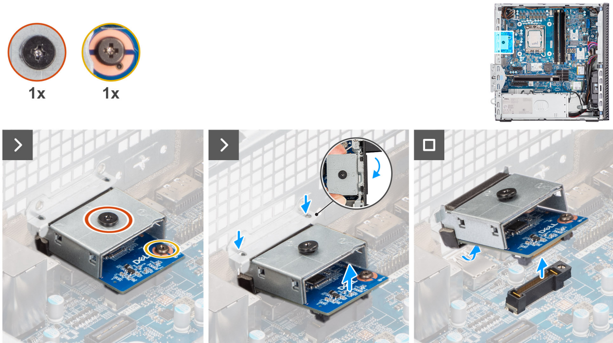
Figure 73. Removing the optional HDMI module
