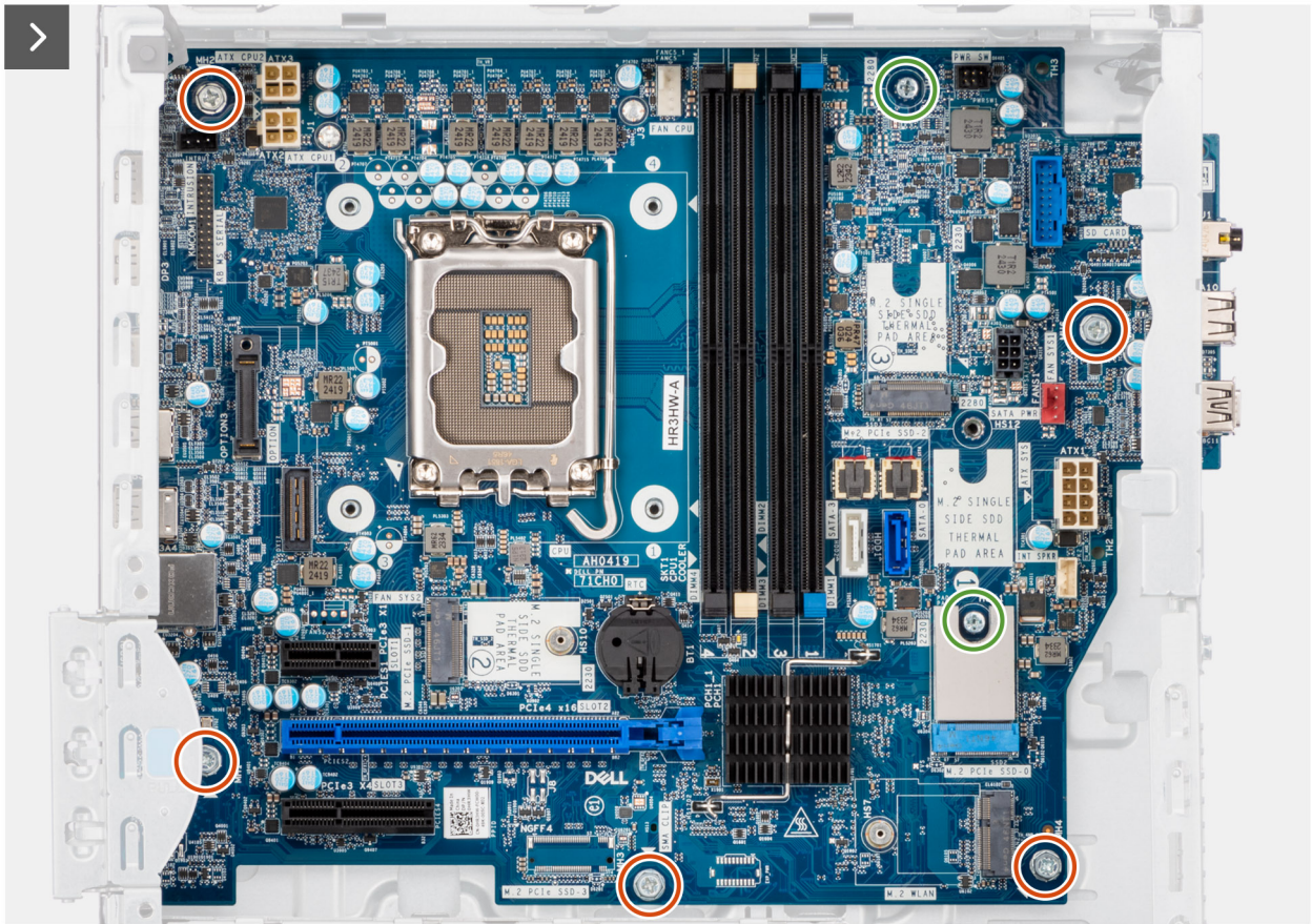
Figure 85. Removing the system board
