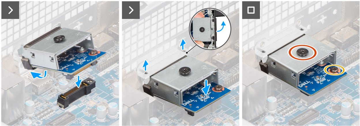
Figure 63. Installing the optional VGA module
