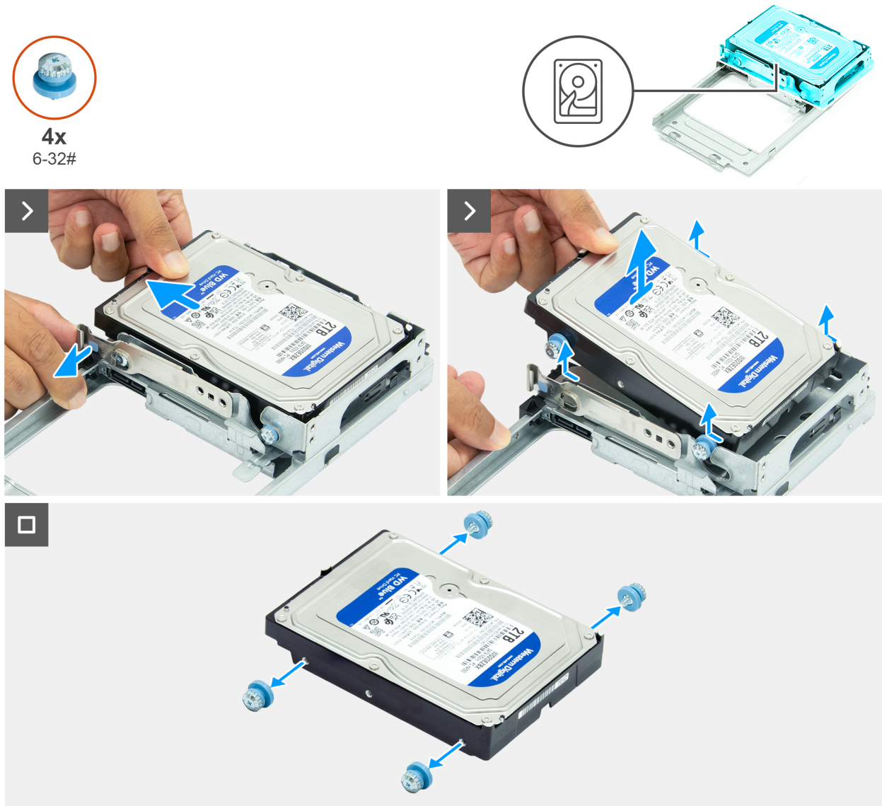
Figure 29. Removing the hard drive
