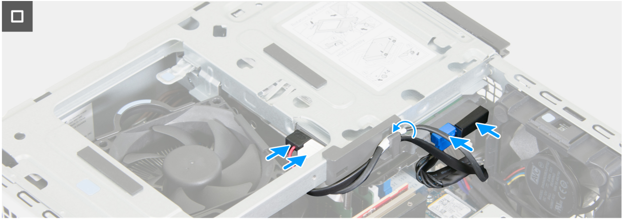
Figure 24. Installing the drive bay
