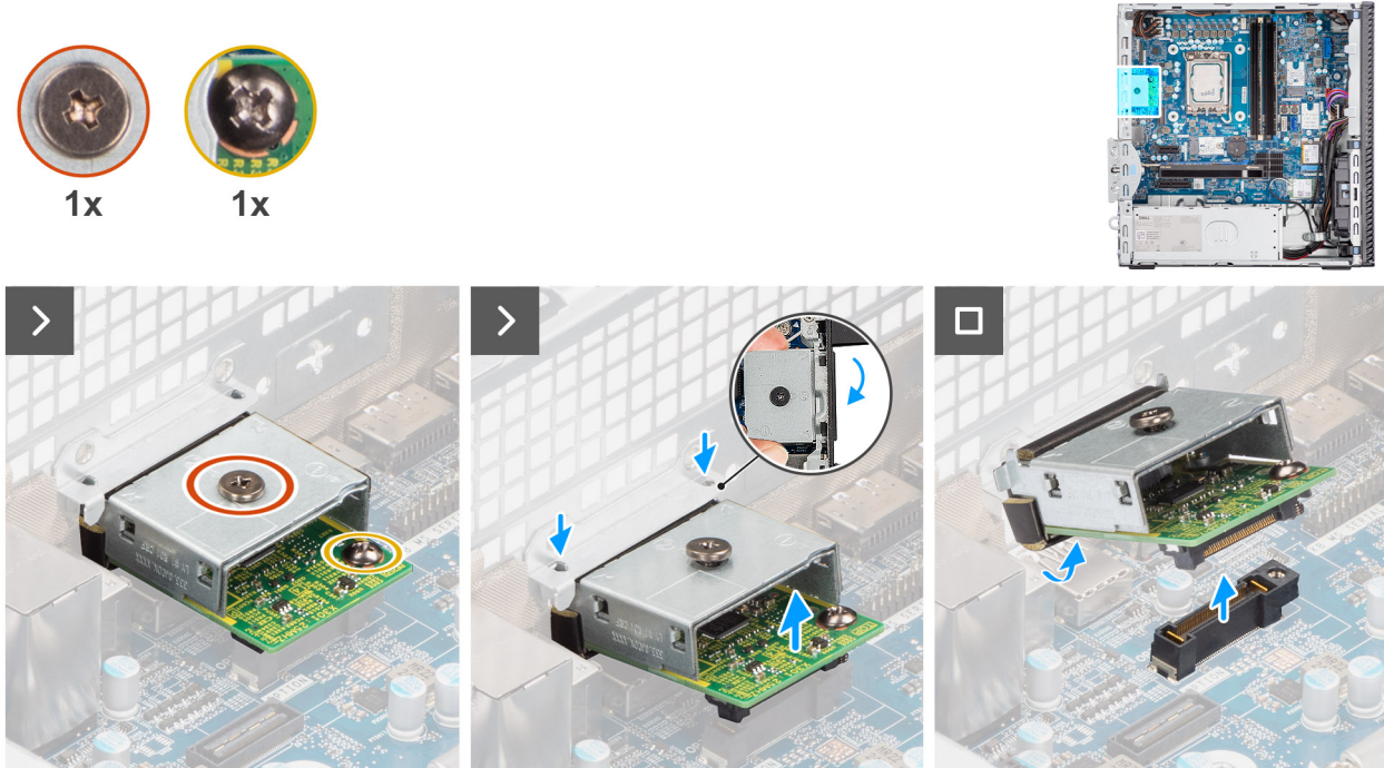
Figure 76. Removing the optional DisplayPort module
