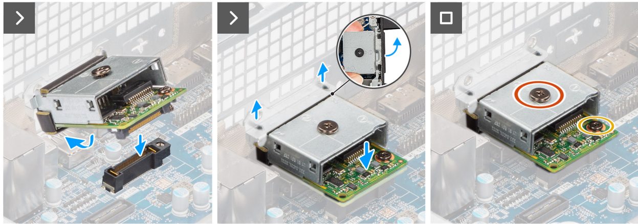
Figure 72. Installing the optional LAN module
