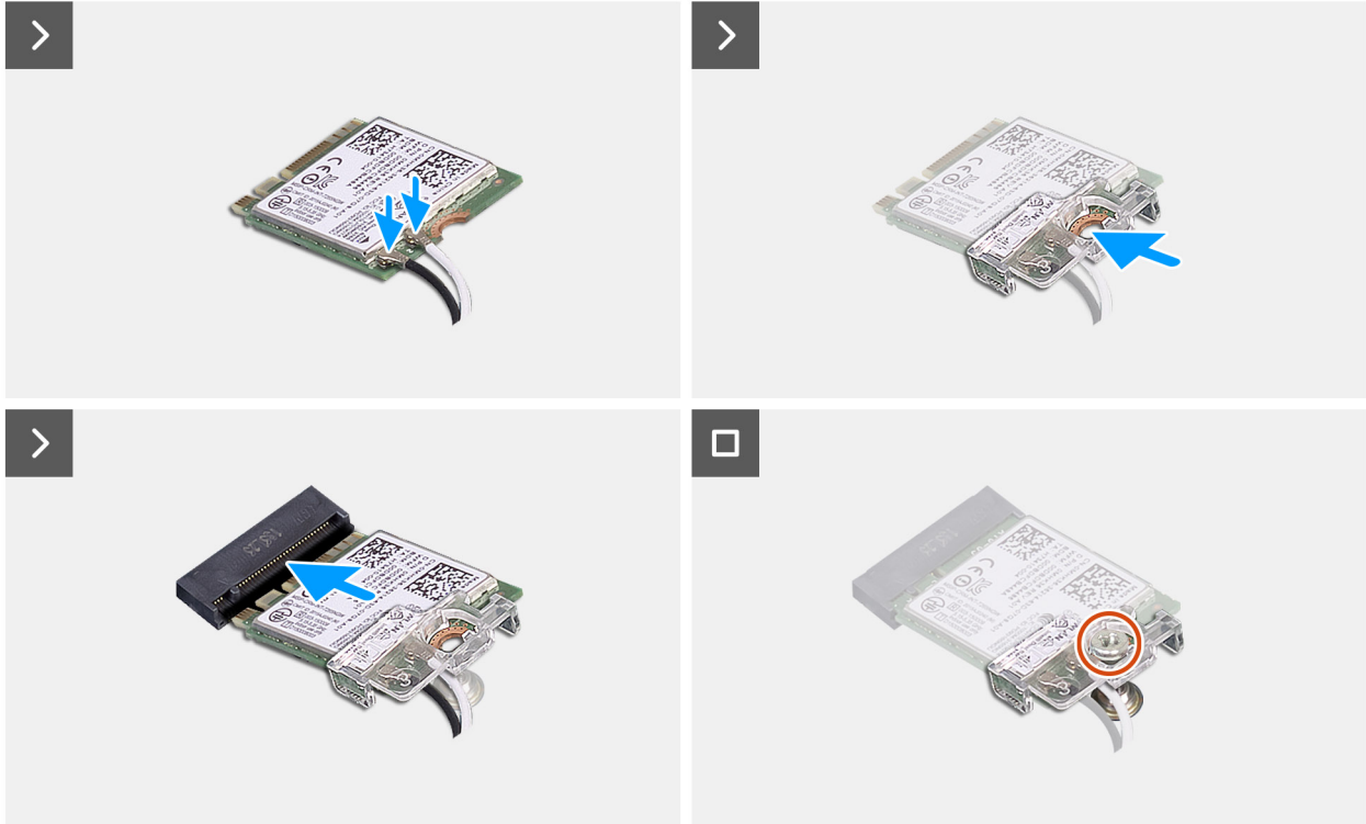
Figure 42. Installing the wireless card
