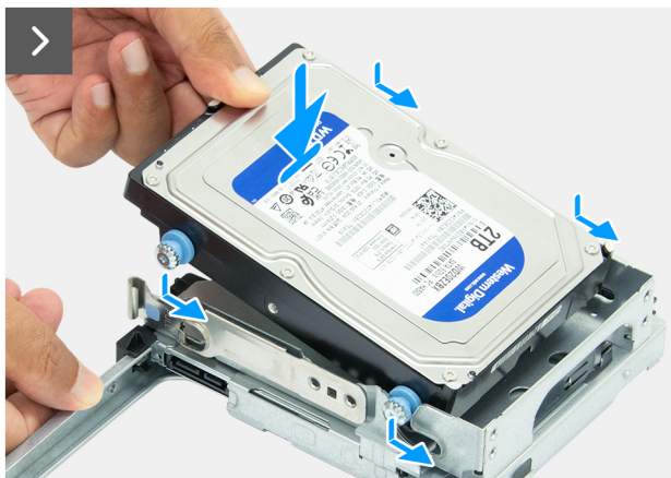
Figure 30. Installing the hard drive
