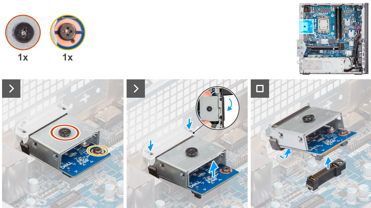
Figure 61. Removing the optional VGA module
