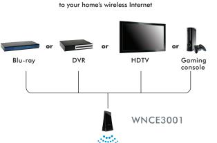
Connect one Ethernet-enabled device
