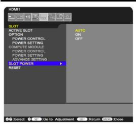
Allows the monitor to supply power to an Option Board slot during power save mode or standby mode.
